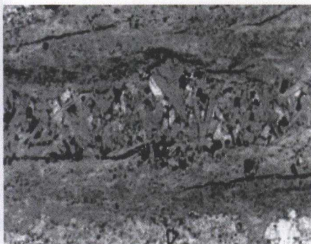
Photo 1: Veinlet of interlocking tourmaline needles, with quartz and chalcocopyrite in altered porphyry. Note vein selvage of fine tourmaline and K-feldspar. El Salvador, Inca Adit level. ppl, Field of view 2.5 mm.
